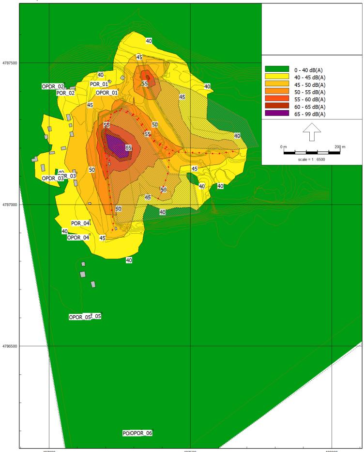
487000 487500 ISO 9613 (1/3-oct.), [Alternative Method 5 - Vertical Expansion + New Footprint - Model1 Noise], Predictor V2022 Licensed to RJ Burnside, Canada
