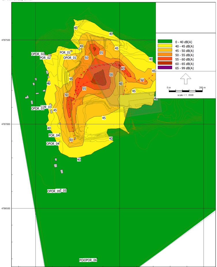
487500 ISO 9613 (1/3-oct.), [Alternative Method 2 - Horizontal - Model1 Noise] , Predictor V2022 Licensed to RJ Burnside, Canada
