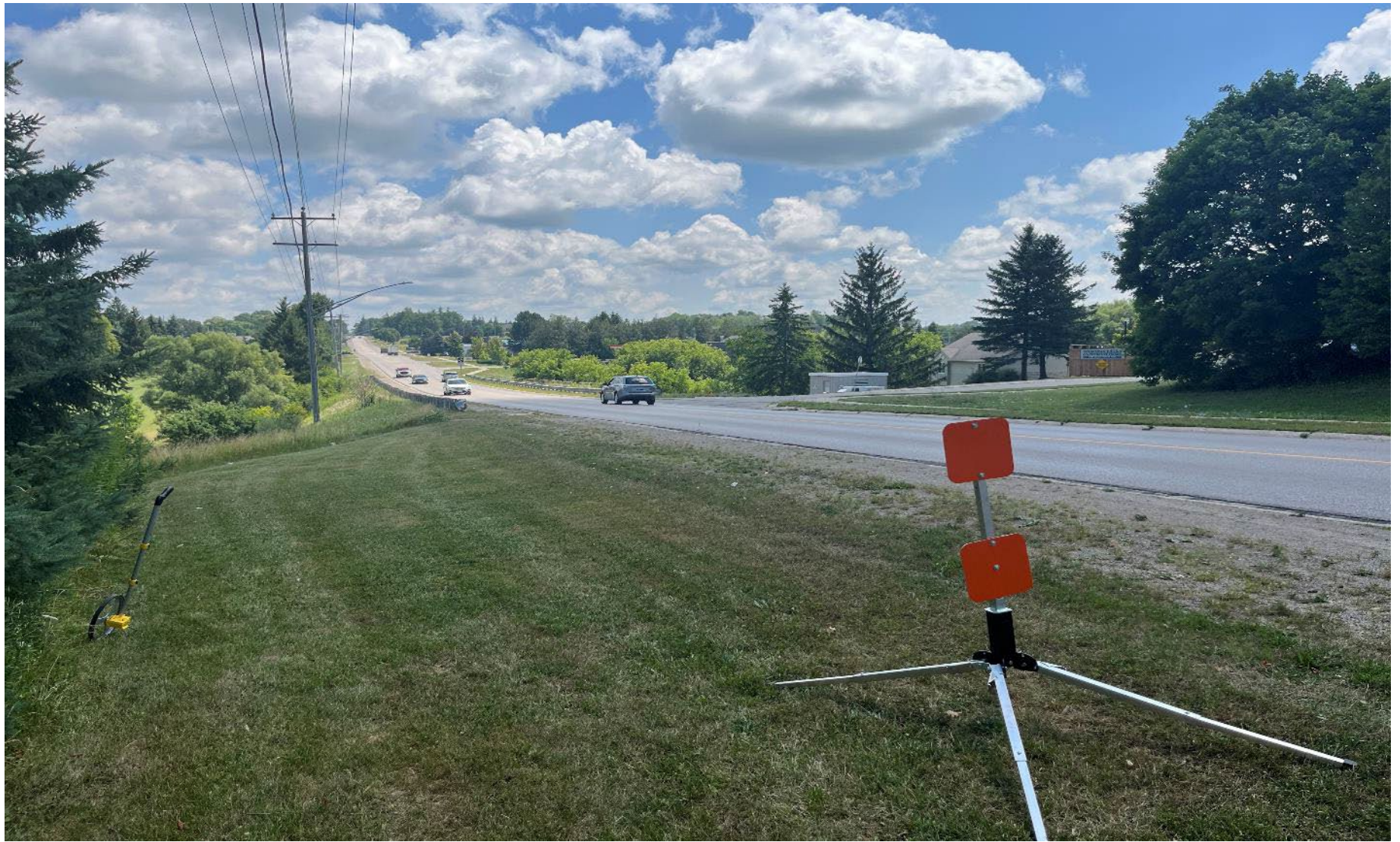
Intersection Sight Distance Right-Turn from Stop (Looking East)
