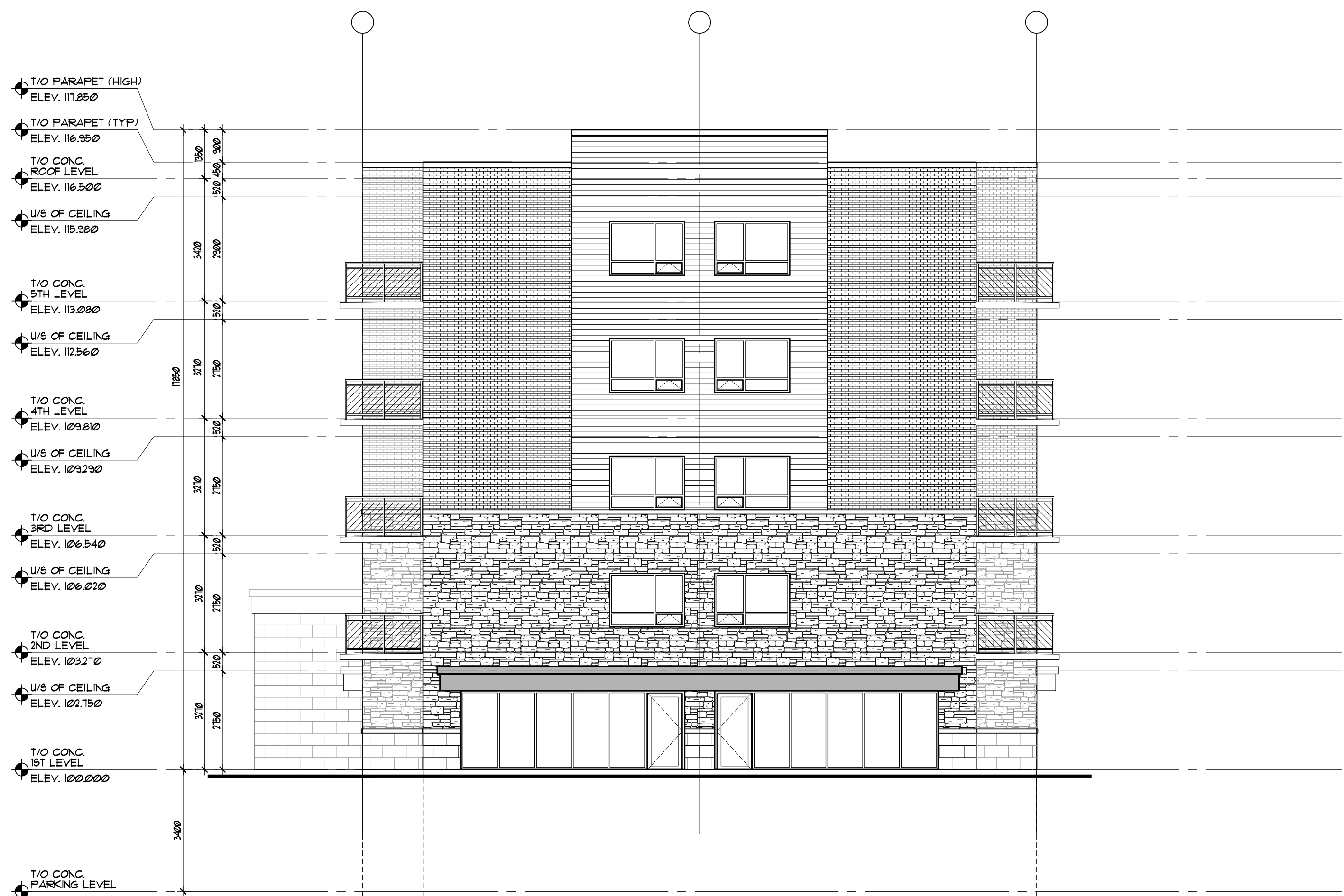
WEST ELEVATION (FACING JAMES STREET)
